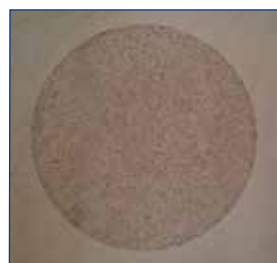
Cross-sections show even distribution of the glass fibers
