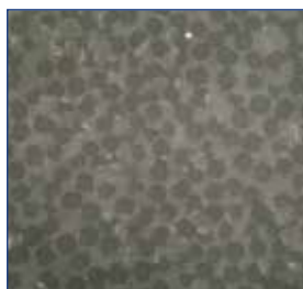
Cross-sections show even distribution of the glass fibers
